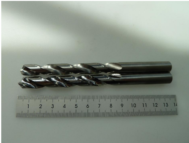
Fig. 3: Drills before and after finishing
