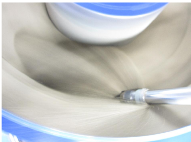
Fig. 2: Drill during finishing
